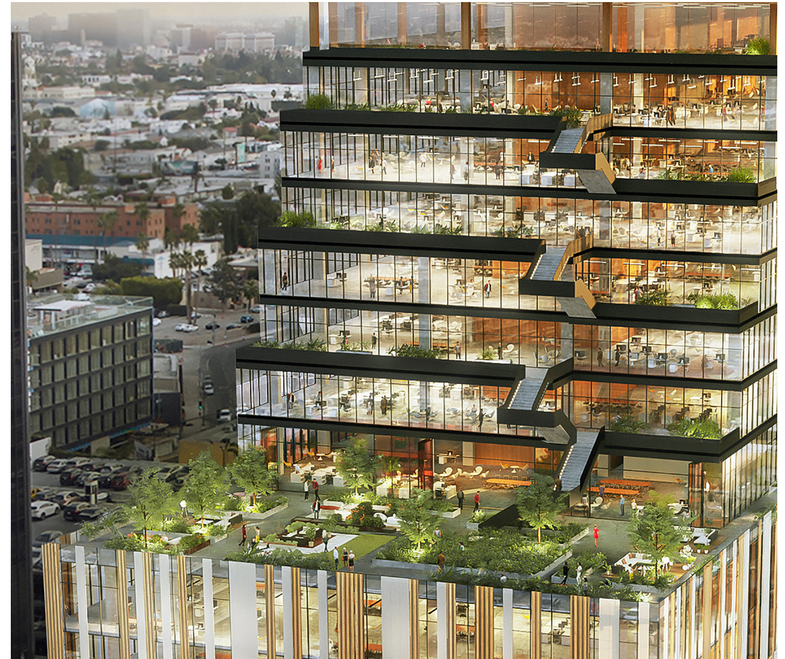
CAMPUS COMMONS AND NORTH TERRACES, SHOWING LARGE DOOR OPENINGS FOR NATURAL VENTILATION, DROUGHT-TOLERANT LANDSCAPING, IRRIGATED WITH RE-USED WATER.
